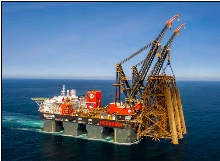
Figure 19. Sleipnir transporting upper Brent Alpha’s upper jacket (Heerema Marine Contractors)
