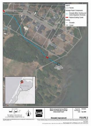
The second location within Harbor District jurisdiction includes clearing and grading of an existing bioswale in MCSD's DMA IV, along the shoreline of the Manila Community Park (Figure 2). Runoff from within DMA IV is generally conveyed from west to east, originating in the Lupin Avenue area to the conveyance system along and under Hwy 255 and crosses Peninsula Drive, the railroad right-of
